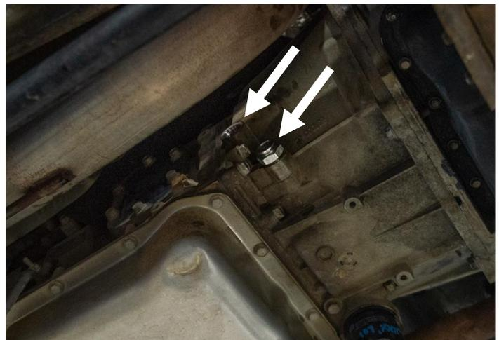
**STEP 14:** Install two of the 7/8"-14 O-ring to -10AN fittings into the "To Cooler" and "From Cooler" ports on the transmission.
