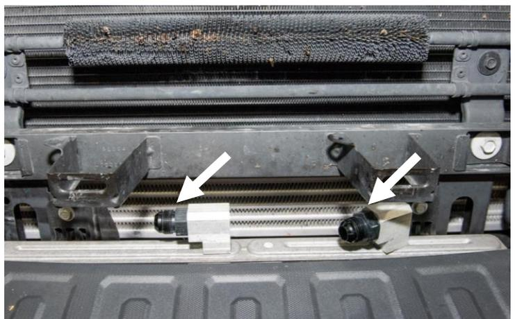
**STEP 12:** Assemble the large flat washers onto two of the 7/8"-14 O-ring to -10AN fittings.
