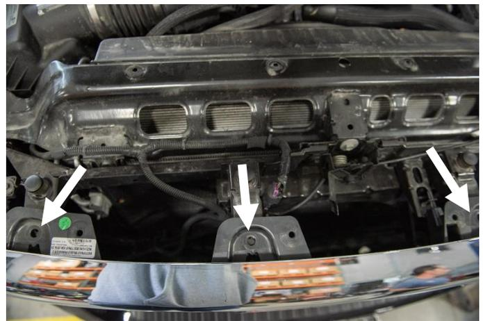
**STEP 4:** Using a long pry bar, release the lower retaining clips for the front grill.
