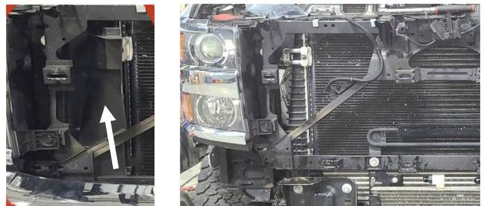
**STEP 6:** To allow for removal of the existing OE lines and installation of the new lines remove the passenger side fender liner.
