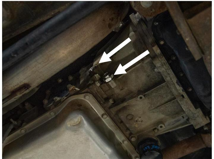
**STEP 9:** With the OE transmission lines removed from the truck, use a 1 1/8" back up wrench and 1 1/4" socket or wrench to remove the factory fittings from each side of the transmission cooler.
