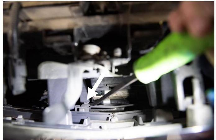
**STEP 5:** Remove the passenger side air deflector located between the core support and radiator.
