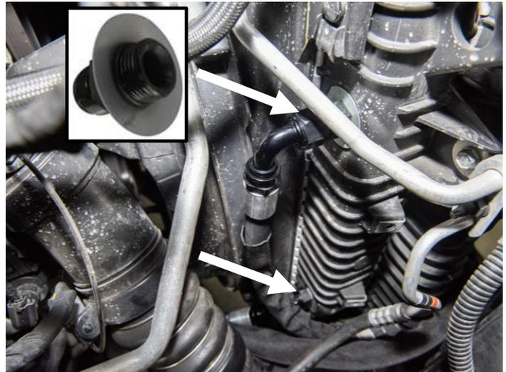
**STEP 13:** Remove the two OE fittings from the transmission using a 1 1/4" socket or wrench.
