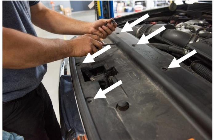
**STEP 3:** Remove the front grill retention bolts located along the top of the grill.
